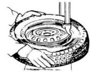
Repeat the above operation for mounting the tyre up bead. (Fig 7)
