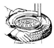
To avoid any damage on type, lubricate the tyre bead and the wheel rim with the lubrication recommended by manufacturer. Put on the tyre and check the situation.
