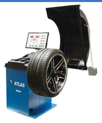
Luxury features are included as standard with the WB49, such as Split-Weight Function for discreetly locating the weights behind the spokes, and an automatic LED light to illuminate the inside of the rim when applying the weights. 2D data entry automatically inputs Offset and Diameter, while the option of 3D input on this model will the also input Width.
